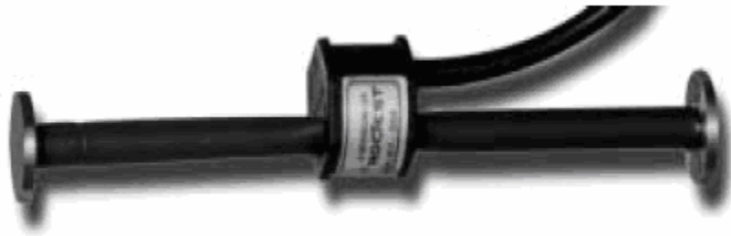
Figure 5 Vibrating Wire Gage EM-5.
